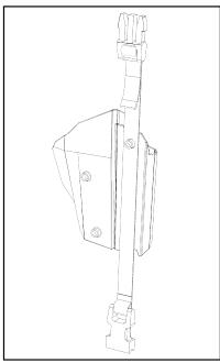
2. Align the Magazine Strap's stitched hole over the forward upper hole on the back side of the Pistol Holster, once again paying attention to the buckle orientation
