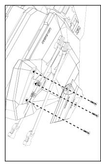
3. Secure the Pistol Holster and Magazine Strap onto the ICOS 2 Body using 3 Torx Head Screws. The Magazine Strap is sandwiched between the Pistol Holster and the ICOS 2 Body. Tighten until snug. Repeat for opposite side.
