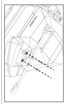
1. Paying attention to the orientation of the buckle, place the Gun Holster Strap with two grommets over the two rearward holes in the side of the ICOS 2 Body using 2 Torx Head Screws. Tighten until snug.
