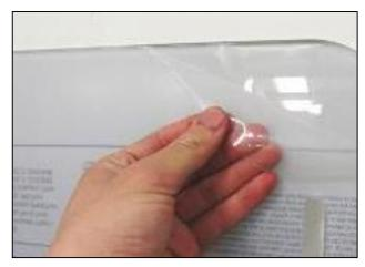
**1.** Peel the plastic fil back from all edges and holes of the windshield before beginning. Remove after windshield is fully installed.
