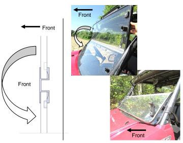
**2. NOTE: The orientation of gasket and parts are very important. See above.** The hinge will ONLY allow the windshield to fold down flat in one direction.
