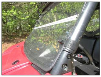
**13.** Place the windshield on the clamps and roll cage of the vehicle. Attach the male rubber plug and plastic spacer on the windshield in the order shown in the next step. It may be helpful to use a small object to push the bolt to the bottom of the plug.
