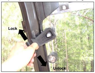
**15.** Rotate both levers perpendicular to the roll cage to lock the windshield in place. To release the top section of the windshield, rotate the lever 90°.
