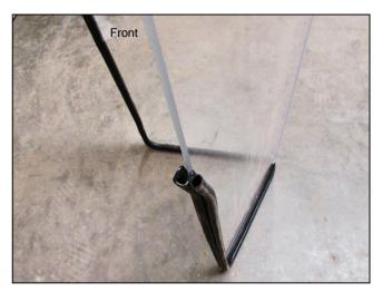
**5.** Press the channel of the gasket into the windshield. The bulb of the gasket should be facing the back of the windshield. It may help to use a rubber mallet to tap on the back of the gasket channel.
