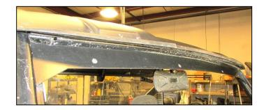
**10.** Place the header panel assembly on the windshield plane of the vehicle near the roof. The brackets should be facing the inside of the vehicle.
