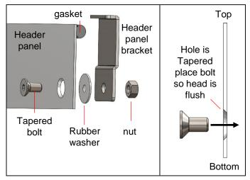
**9.** Insert the tapered bolt into the countersunk side of the hole. The adhesive gasket should be on the same side as the brackets. Loosely attach the header panel brackets with the tapered bolts, nut and washer.
