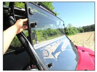
**16.** Push the top half of the windshield down and firmly press the two rubber plugs against each other to lock windshield in down position.
