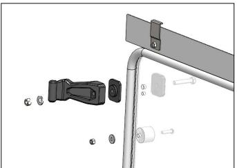
6. Attach the Lever using the inner and outer windshield mounting plates. The lever should be tight enough to just be able to turn with some force. The lever should be on BACK of the windshield.
