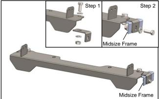
**NOTE: Follow these instructions for the MIDSIZE ranger** Step 1. Hand tighten (2) M8x20mm bolts, washers and locknuts to secure the Midsize Adapters (J) to the bumper mount. Step 2. Place bumper mount with adapter brackets on the midsize bumper. Line up the holes on the Midsize frame and secure with (2) M8x20mm bolts. Tighten all 4 fasteners. Skip this step if you have a full size ranger.
