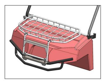
8. Attach the riser assembly to the front of the hood rack and bolt the two front riser caps in place. Snug the cap bolts, but keep them loose enough to allow rotation. Make sure all 4 clamps are open, then set the rack in place.
