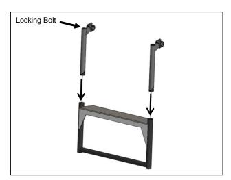
7. Note the riser orientation shown above. Insert the 2 Front riser stems (H) into the front riser/light mounting plate a few inches in. Tighten the locking bolt at the top of the tube with allen wrench just enough to hold the riser stems in place. You will tighten after final assembly.
