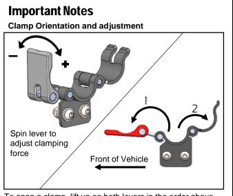
To open a clamp, lift up on both levers in the order above. Orient all clamps so the first clamp lever opens towards the front of the vehicle. To increase clamping force, spin the lever clockwise; to decrease the clamping force, spin the lever counter-clockwise before locking.
