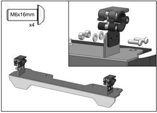
3. Attach the two front clamps (D) to the bumper mount (C) using (4) M6 x 16mm bolts, (2) washers and (4) locknuts. Make sure all clamp levers open away from the vehicle.
