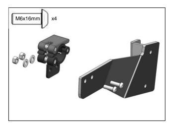
6. Attach the two Rear Clamps (E) To the Hood Rack Bracket (F) with two M6 x 16mm socket head bolts, 4 washers and 2 nuts. The clamp lever should open towards the front of the vehicle.
