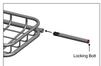
2. Insert the two (G) Extendable Tubes in the ends of the hood rack. Tighten bolts at the ends with a 6mm Hex key just enough to hold tube in place. You will tighten after final assembly.
