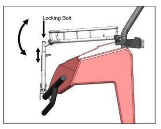
9. Adjust the width of the extendable tubes (G) so they stick out just past the clamps. The hood rack angle can be adjusted by loosening the bolt on the front riser stems and lifting up or pushing down on the front of the rack. Adjust clamps and brackets as necessary, then tighten all bolts. We recommend no more than 5% of slope to the hood rack.
