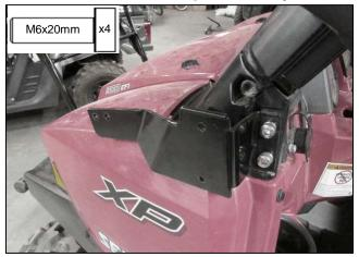
5 Attach the hood rack brackets (F) to the sides of the roll cage using (4) M8 x 20mm socket head bolts as shown above.
