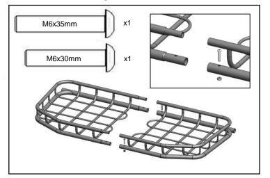
1. Assemble two sides of rack. Secure the back of the rack with a single M6 35mm Socket Head bolt and lock nut. Secure the front of the rack with a single M6 30mm Socket Head bolt and lock nut.
