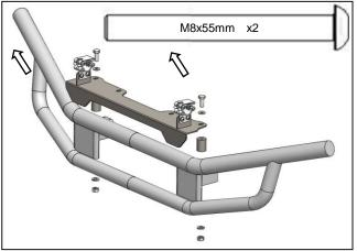
4. Set the two 1" spacers on the bumper holes. Then set the mount on the bumper and attach using (2) M8 x 55mm Hex Bolts, two 1" Spacers (J), six washers, and two M8 Lock Nuts. The order is shown in the picture above.
