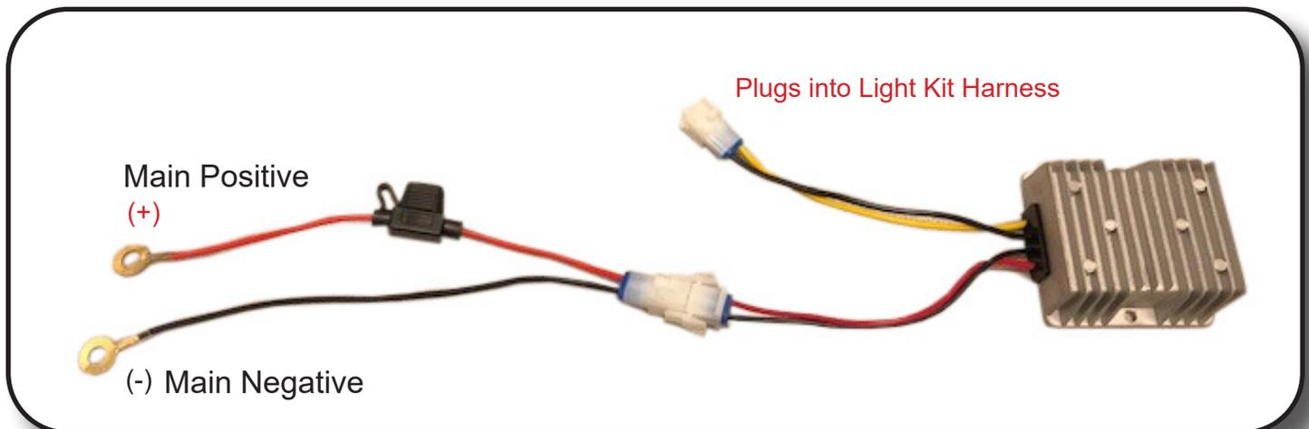
The voltage converter included must be used on all carts electric and gas. Connect the red wire with the fuse to the main positive terminal of the battery pack. Connect the black wire to the main negative terminal of the battery pack and tighten hardware.
