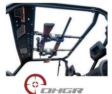
The OHGR (OverHead Gun Rack) installs between the factory header panel up front and the ROPS (rollover protection system) in the rear. The OHGR stores the guns overhead and out of the way. The OHGR (pronounced 'ogre') looks as good as your guns—not like something someone made in the garage.
