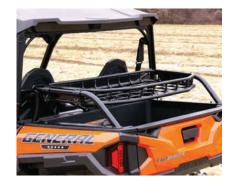
Secure and carry cargo above the dump bed of your General. The basket measures 42" x 20" and sits 4.5" above the dump bed edge. Side rails are 9" tall and there is a 100 lb weight limit.
