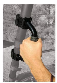
The most stable removable UTV Grab Handle on the market! SEIZMIK's grab handle is an extremely durable solution for adding a stable grip to your UTV. Rubber pads keep it from sliding and twisting while driving through the roughest terrain or entering and exiting the UTV.
