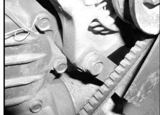
Figure 12b-14 Alternator Mounting Bolt
