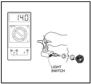
Figure 11b-37 Light Switch Test
