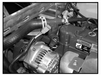
Figure 11b-31 Thermostat Switch Connector
