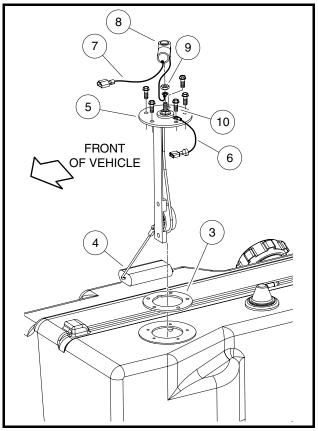
Figure 13b-15 Fuel Level Sending Unit Removal
