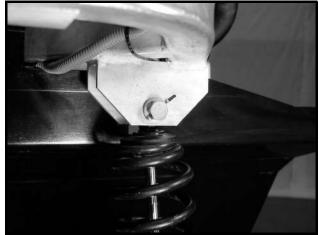
Figure 14-2 Upper Shock Absorber Bolt
