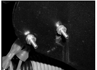
Figure 12b-8 Reverse Warning Buzzer Limit Switch Adjustment Slot
