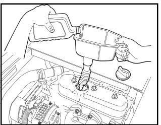
Figure 10-12 Add Engine Oil – Gasoline Vehicles
