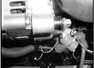
Figure 12b-12 10-Gauge Red Wire at Alternator
