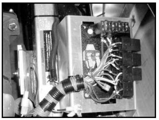
Figure 11b-5 Electrical Component Mounting Plate
