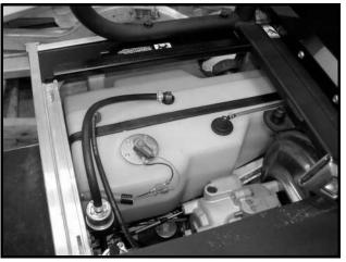
Figure 13b-18 Diesel Fuel Tank
