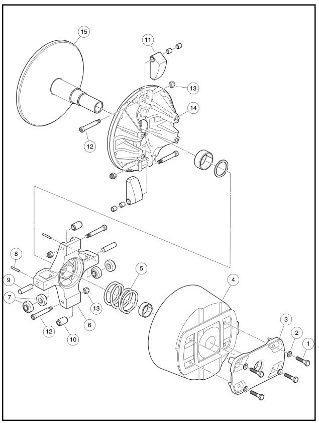
Figure 13b-37 Drive Clutch Assembly
