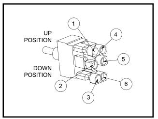
Figure 11a-35 Bed Lift Switch Terminals
