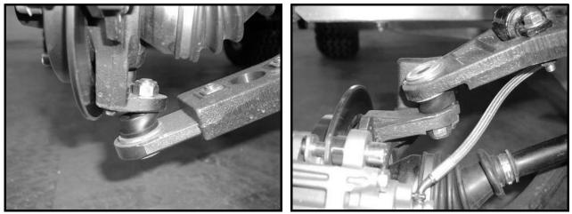
Figure 7-27 Lower Ball Joint
