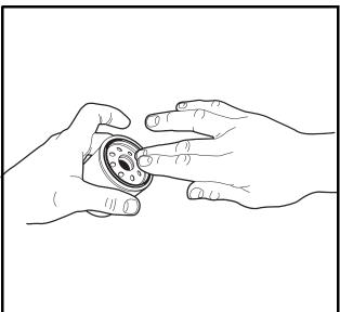
Figure 10-11 Coat Rubber Seal
