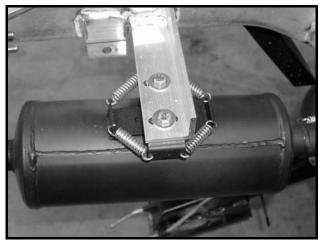
Figure 13b-11 Muffler and Bracket
