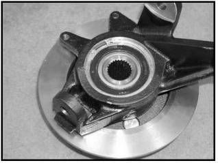
Figure 6-16 Upright, Bearing and Shaft Assembly
