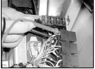
Figure 11b-12 Start Relay Contact Test
