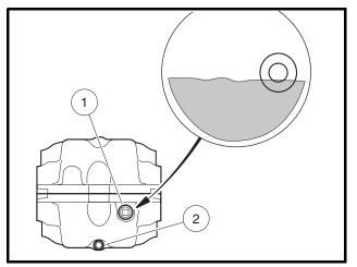
Figure 10-18 Rear Differential Lubrication Level
