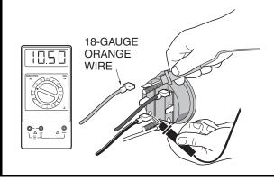
Figure 11b-36 Fuel Gauge Voltage Test
