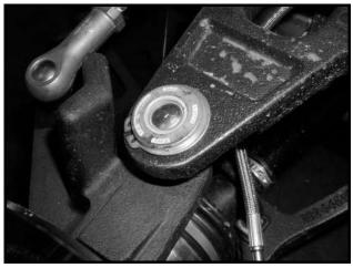
Figure 7-31 Ball Joint C-Clip
