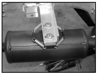
Figure 13a-3 Muffler and Bracket
