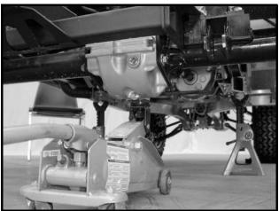
Figure 14-16 Position Floor Jack Under Differential
