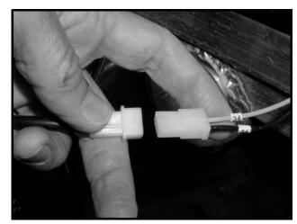
Figure 14-10 Differential Clutch Connector
