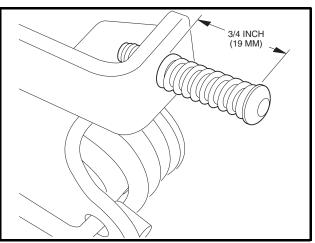
Figure 5-3 Ground Speed Set Screw Adjustment
