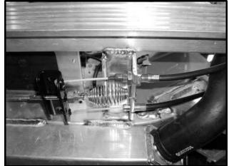
Figure 6-23 Park Brake Frame Bracket
