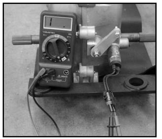
Figure 11a-20 Neutral Switch – Reverse Position
