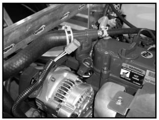
Figure 12b-16 Thermostat Switch
