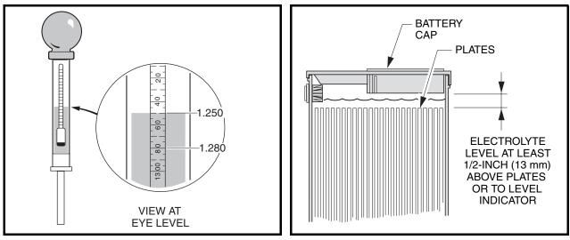
Figure 11a-3 Hydrometer Test
