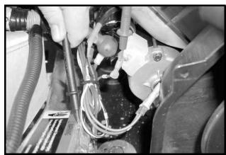
Figure 11a-10 Solenoid Coil Wire (w58) Removed
