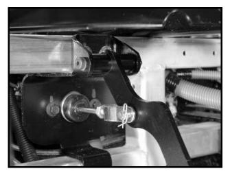
Figure 6-21 Master Cylinder Rod and Brake Pedal
