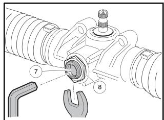
Figure 7-18 Rack and Pinion Adjustment
