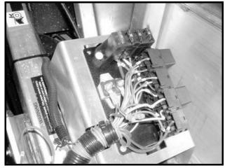
Figure 11b-24 Differential Relay Removed
