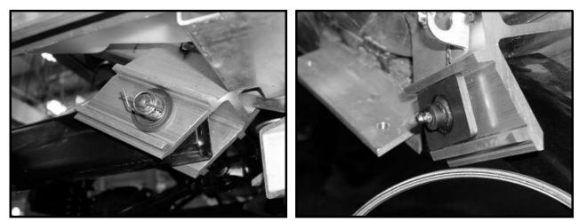
Figure 9-3 Swing Arm Bolt, Nut and Rue Pin
