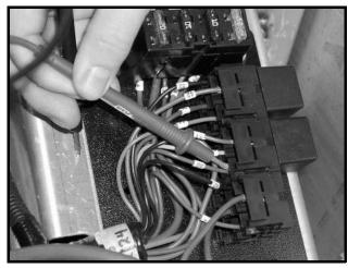
Figure 11a-14 Differential Relay Coil Circuit Test
