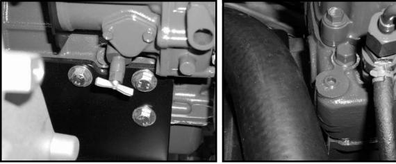
Figure 15-1 Engine Block Coolant Drain Valve
