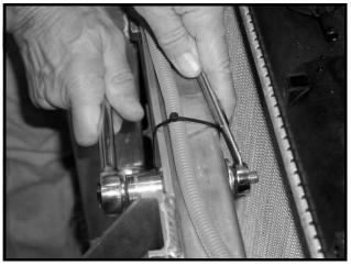
Figure 15-11 Top Front Frame Bolts
