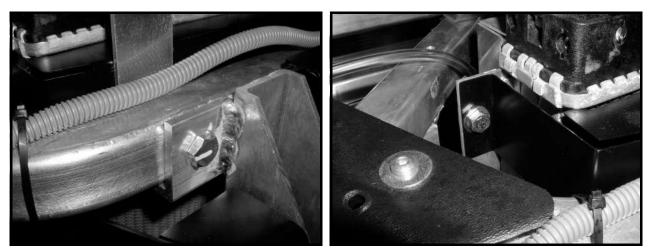
Figure 15-9 Radiator Bracket Front Frame Mount
