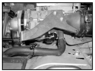
Figure 13a-26 Choke Cable on Engine
