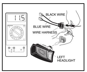
Figure 11b-38 Voltage Measurement at Headlight Socket
