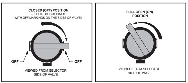
Figure 13a-10 Closed Fuel Shut-Off Valve
