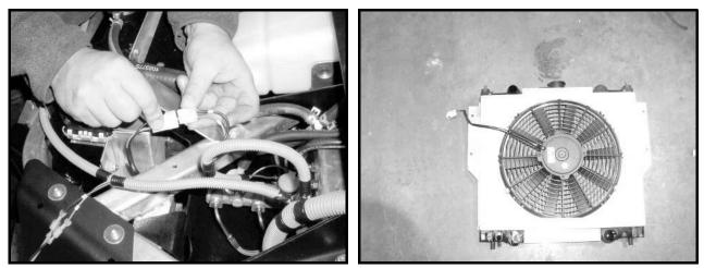
Figure 12b-17 Fan Motor Connector
