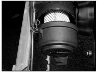
Figure 13b-29 Air Filter Cartridge
