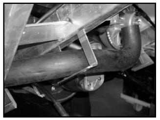
Figure 13b-31 Air Intake Support Bracket
