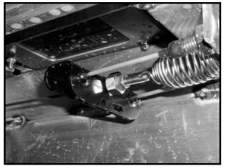
Figure 5-6 Park Brake Adjustment Nuts
