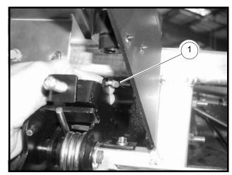
Figure 13b-20 Z-Shaped Cable End
