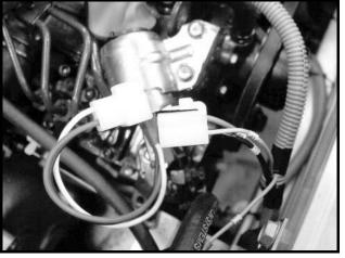
Figure 11b-25 Fuel Solenoid Three-Pin Connector
