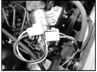
Figure 12b-3 Fuel Solenoid Three-Pin Connector
