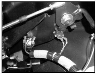
Figure 11a-25 Reverse Warning Buzzer and Limit Switch
