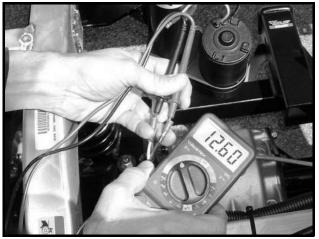
Figure 11b-40 Bed Lift Motor Voltage Reading with Switch in UP position
