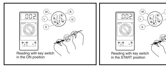
Figure 11a-8 Key Switch Test – Accessory Terminal
