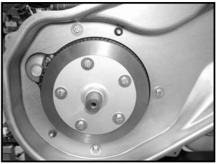
Figure 13b-40 Inner Cover Hardware on Diesel Engine
