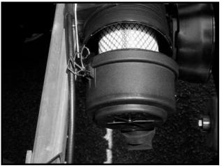
Figure 13a-25 Air Filter Cartridge
