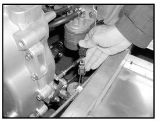
Figure 11a-17 Neutral Switch Two-Pin Connector
