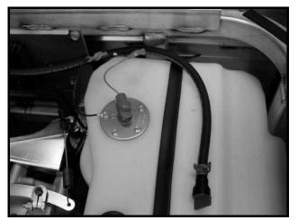
Figure 13a-8 Gasoline Fuel Tank
