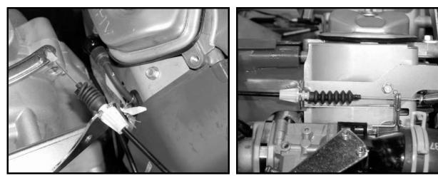
Figure 13a-19 Governor Cable on Transmission
