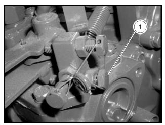
Figure 13b-27 Idle Throttle Adjustment Screw
