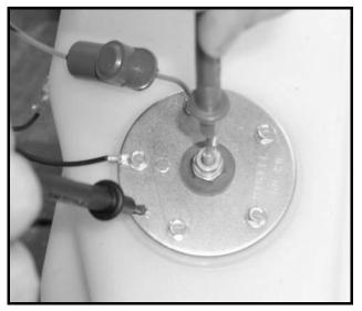
Figure 11b-34 Fuel Level Sending Unit Test
