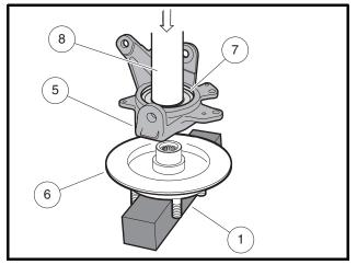
Figure 6-15 Press Disc and Hub into Bearing
