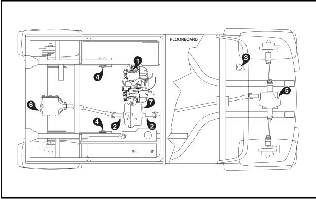
Figure 10-1 Lubrication Points – Gasoline Vehicles
