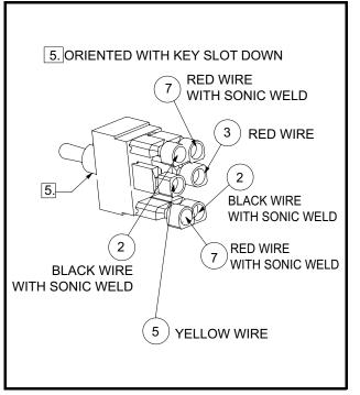
Figure 12b-19 Bed Lift Switch Wiring
