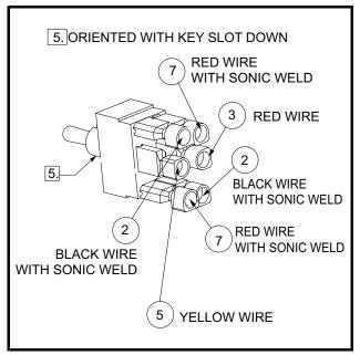
Figure 12a-11 Bed Lift Switch Wiring
