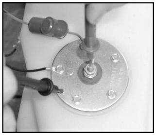
Figure 11a-27 Fuel Level Sending Unit Test
