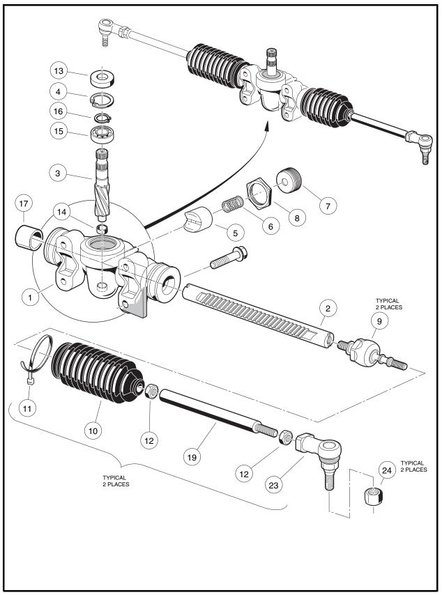
Figure 7-16 Steering Gear Assembly
