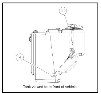
Figure 13b-17 Fuel Level Sending Unit Position
