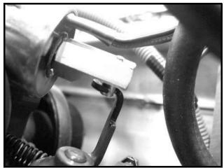
Figure 12b-4 Fuel Solenoid Lever
