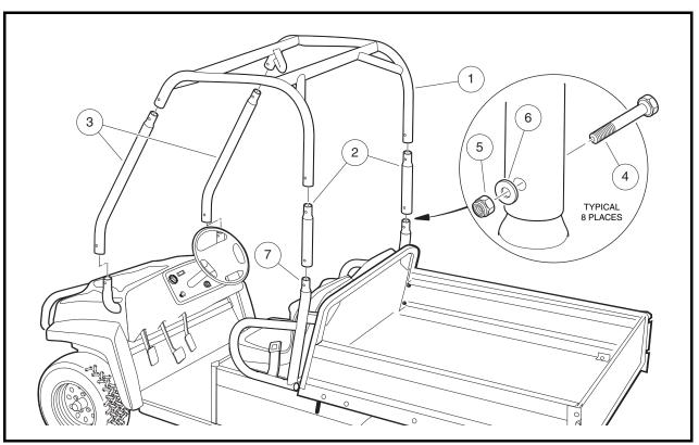
Figure 4-4 Roll-Over Protective Structure (ROPS)
