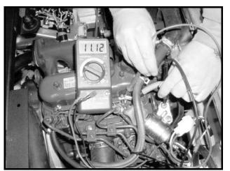
Figure 11b-32 Glow Plug Circuit Test
