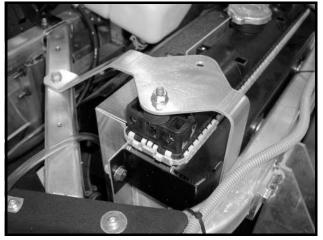
Figure 15-7 Radiator Bracket Attachment
