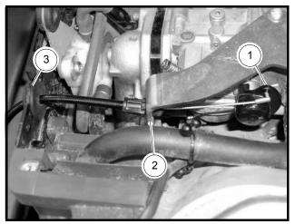
Figure 4-3 Engine Choke Cable at Engine (Gasoline Vehicles)
