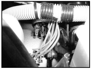
Figure 11b-23 Disconnected Multi-Pin Connector at Key Switch
