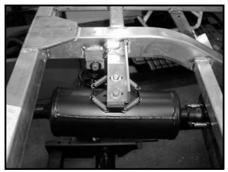
Figure 13a-2 Muffler Bracket and Inlet Pipe
