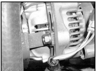
Figure 12b-13 Belt Tension Adjustment Bolt
