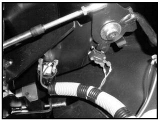
Figure 12a-6 Reverse Warning Buzzer and Limit Switch
