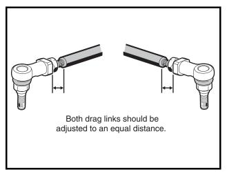
Figure 7-25 Adjust Both Drag Links
