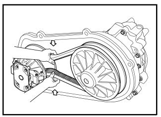
Figure 13b-35 Drive Belt Removal
