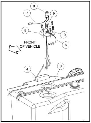
Figure 13a-5 Fuel Level Sending Unit Removal
