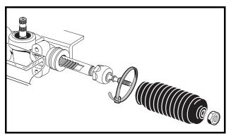
Figure 7-9 Dust Bellows Clamp
