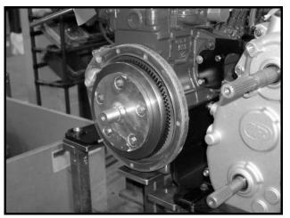
Figure 13b-42 Diesel Inner Cover Spacer
