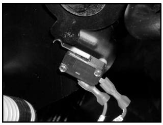
Figure 12a-8 Reverse Warning Buzzer Limit Switch (Properly Adjusted)
