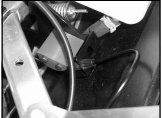
Figure 13b-21 Accelerator Cable Pedal Bracket (Diesel Vehicles)
