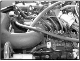
Figure 13b-2 Fuel Return Line at Relief Valve
