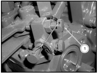
Figure 13b-28 High-Speed Throttle Adjustment Screw
