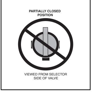
Figure 13a-12 Incorrect Fuel Shut-Off Valve
