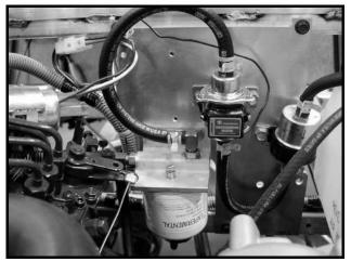
Figure 13b-12 Fuel Filters and Fuel Pump
