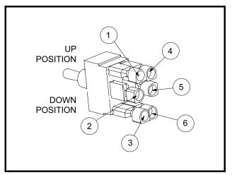
Figure 11b-42 Bed Lift Switch Terminals
