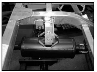
Figure 13b-9 Muffler Bracket and Inlet Pipe
