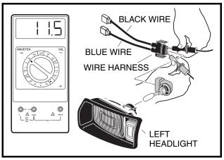
Figure 11a-31 Voltage Measurement at Headlight Socket
