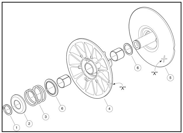
Figure 13a-36 Driven Clutch Assembly
