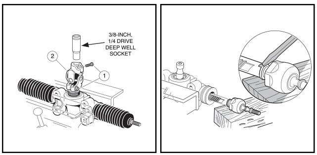
Figure 7-19 Adjust Rack and Pinion Resistance
