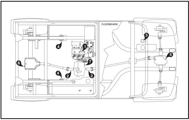
Figure 10-2 Lubrication Points – Diesel Vehicles
