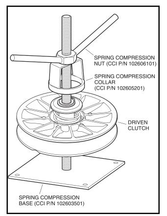
Figure 13a-35 Driven Clutch Service Tools
