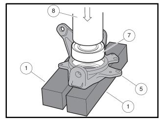
Figure 6-14 Position Upright for New Bearing
