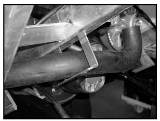
Figure 13a-28 Air Intake Support Bracket
