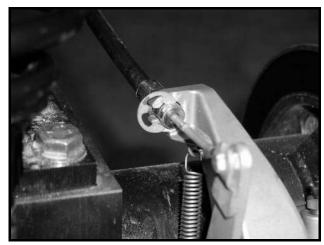
Figure 6-22 Park Brake Cable Attachment
