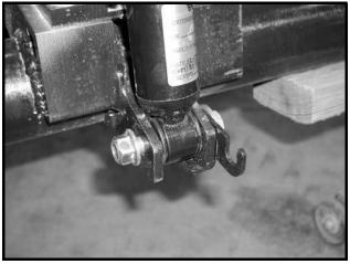
Figure 9-2 Remove Lower Driver-Side Shock Bolt
