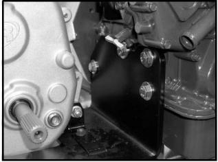
Figure 13b-8 Transmission Side Diesel Engine Mount
