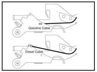
Figure 13a-16 Z-Shaped Cable End in Hole at Pedal
