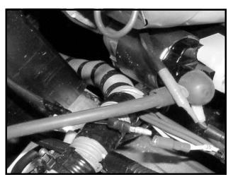
Figure 11a-16 Carburetor Coil Bullet Connector
