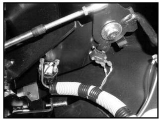
Figure 12b-7 Reverse Warning Buzzer and Limit Switch
