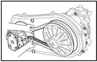
Figure 13a-32 Drive Belt Removal
