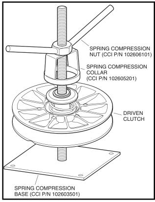
Figure 13b-38 Driven Clutch Service Tools
