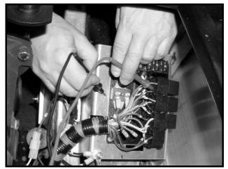
Figure 11b-11 Start Relay Coil Circuit Test
