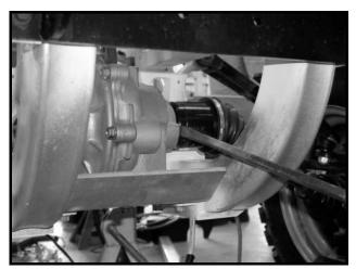
Figure 14-5 Separate Half Shaft from Differential
