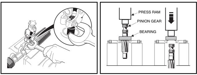
Figure 7-12 Remove Pinion from Housing
