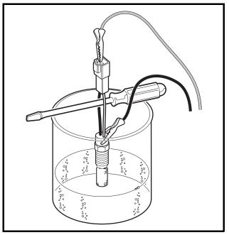
Figure 11b-18 Fan Thermostat Switch Test Setup
