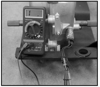
Figure 11b-27 Neutral Switch – Forward Position
