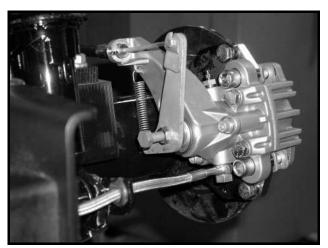
Figure 14-15 Park Brake Cable and Hex-Head Bolts
