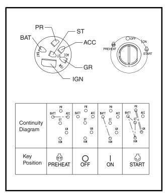
Figure 11b-8 Key Switch Terminals and Continuity Diagram
