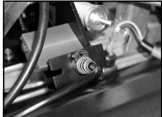
Figure 13a-14 Accelerator Cable Pedal Bracket (Gasoline Vehicles)
