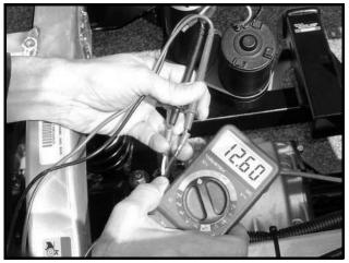
Figure 11a-33 Bed Lift Motor Voltage Reading with Switch in UP position
