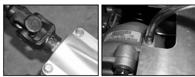
Figure 14-8 Roll Pin in Front Drive Shaft
