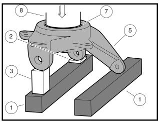
Figure 6-13 Position Upright for Bearing Removal
