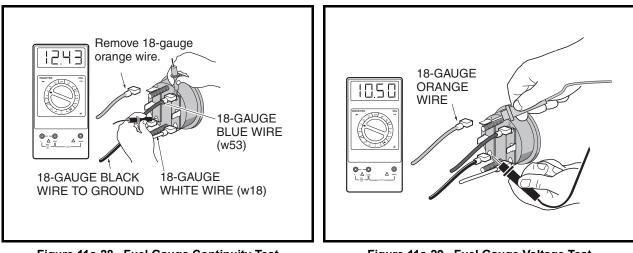
Figure 11a-28 Fuel Gauge Continuity Test
