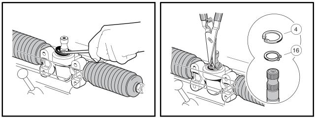
Figure 7-10 Remove Dust Seal
