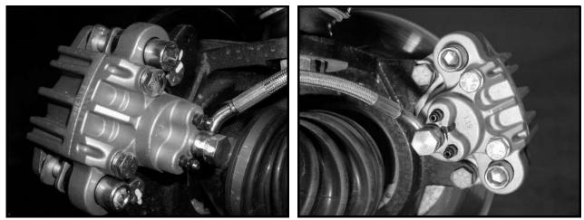
Figure 6-3 Front Brake Pad and Caliper
