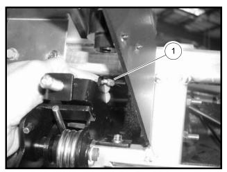
Figure 5-1 Z-Shaped Cable End – Gasoline Vehicles
