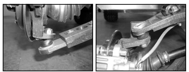
Figure 6-9 Lower Ball Joint and Upright
