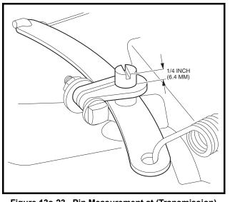
Figure 13a-23 Pin Measurement at (Transmission) Governor Arm
