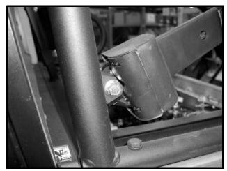
Figure 4-5 Coiled Seat Belt Assembly
