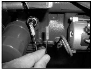
Figure 13b-5 Thermostat Switch Wire Connector
