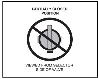
Figure 3-6 Fuel Shut-Off Valve – Partially Closed Position
