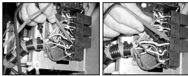
Figure 11b-15 Fan Relay Coil Circuit Test
