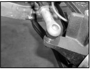
Figure 7-26 Drag Link Ball Joint
