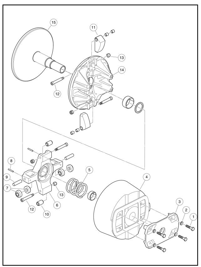
Figure 13a-34 Drive Clutch Assembly
