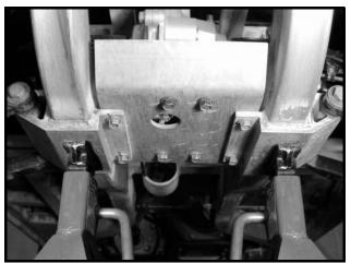
Figure 14-11 Front Differential Plate
