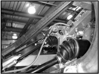
Figure 6-20 Front Brake Line Support Brackets
