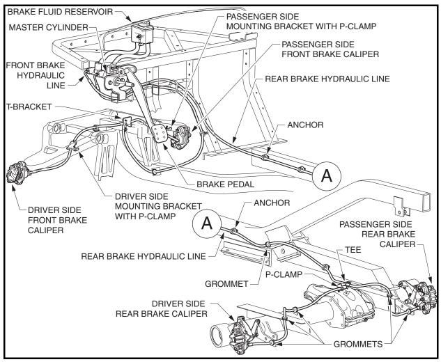
Figure 6-1 Hydraulic Disc Brake System
