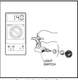
Figure 11a-30 Light Switch Test
