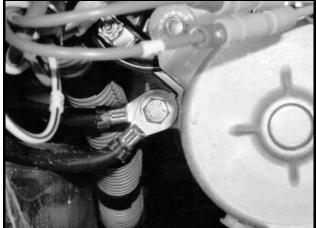
Figure 11a-7 Engine Ground (Under Starter)
