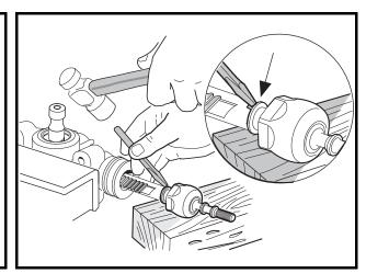
Figure 7-15 Remove Inner Ball Joints
