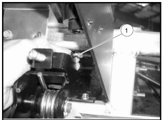
Figure 13a-13 Z-Shaped Cable End (Gasoline Vehicles)
