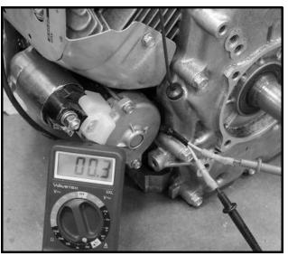
Figure 11a-21 Charge Coil Test (At Voltage Regulator Figure 11a-22 Charge Coil Test (At Bullet Connectors) Multi-Pin Connector)
