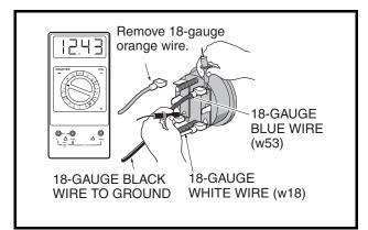
Figure 11b-35 Fuel Gauge Continuity Test
