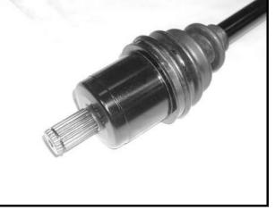
Figure 14-6 Compression Ring on Spline
