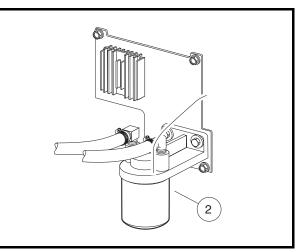
Figure 10-8 Replace Engine Oil Filter – Gasoline Vehicles
