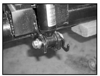
Figure 14-17 Lower Driver Side Shock Mount
