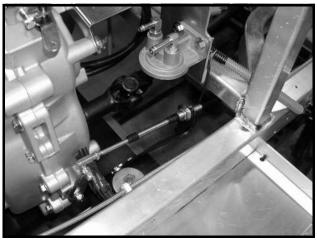
Figure 14-24 Forward/Reverse Shifter Cable at Transmission
