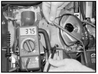
Figure 11a-26 Carburetor Solenoid Coil Resistance
