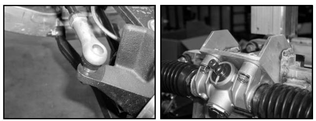
Figure 7-5 Drag Link Ball Joint
