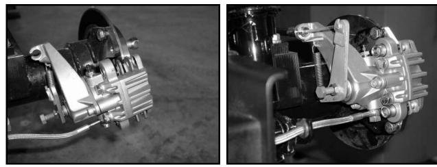
Figure 6-5 Rear Brake Pad and Caliper
