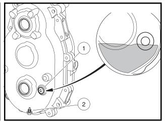
Figure 10-17 Transmission Lubrication Level
