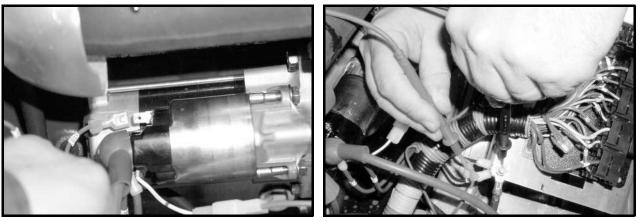
Figure 11b-9 Solenoid Coil Wire (w58) Removed
