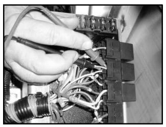
Figure 11b-14 Differential Relay Contact Test
