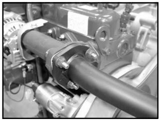
Figure 13b-10 Diesel Manifold Pipe Flange
