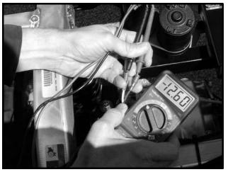
Figure 11a-34 Bed Lift Motor Voltage Reading with Switch in DOWN position
