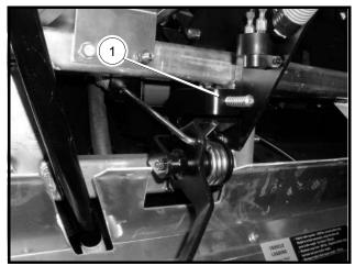
Figure 13a-24 High-speed Adjustment Screw
