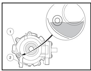
Figure 10-16 Front Differential Lubrication Level
