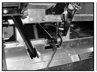
Figure 5-2 Accelerator Pedal Assembly
