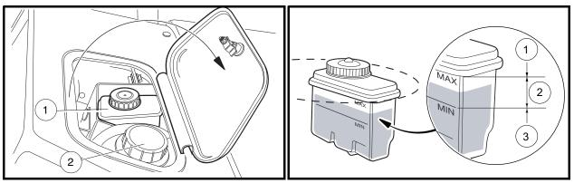
Figure 10-3 Brake Fluid and Coolant Access Door
