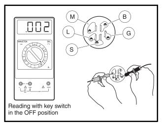
Figure 11a-24 Key Switch Test – Engine Kill Circuit
