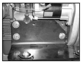
Figure 13b-7 Driver Side Diesel Engine Mount
