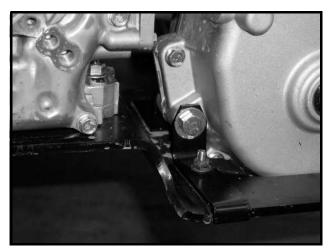
Figure 13a-1 Engine Mounting Bolts
