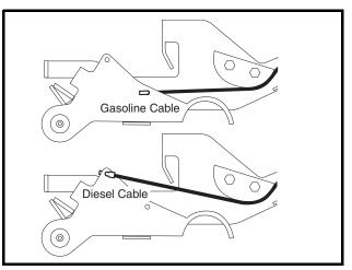
Figure 13b-22 Z-Shaped Cable End in Hole at Pedal
