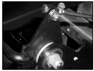
Figure 14-22 Forward/Reverse Shifter Cable at Shift Lever
