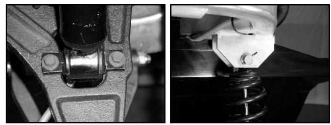
Figure 7-35 Front Shock Bottom Mount
