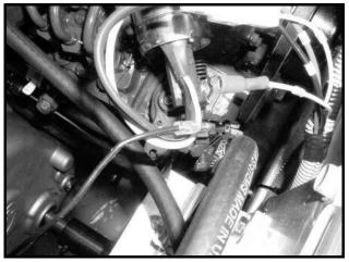
Figure 11b-26 Fuel Pump Bullet Connector
