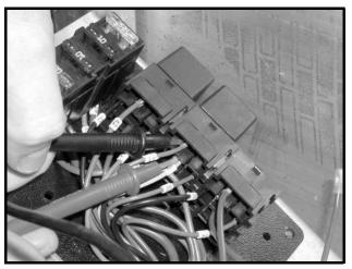
Figure 11a-15 Differential Relay Contact Test
