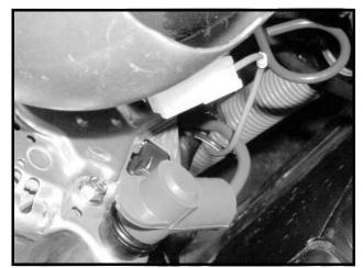
Figure 12b-11 18-Gauge Purple Wire at Alternator
