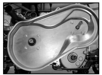
Figure 13a-37 Inner Clutch Cover
