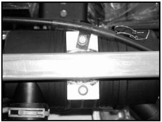
Figure 13a-27 Air Filter Canister
