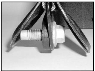
Figure 4-6 Center Seat Belt Fastener
