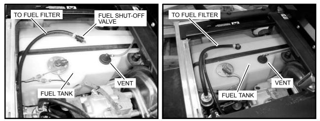
Figure 3-2 Fuel Tank – Gasoline Vehicles
