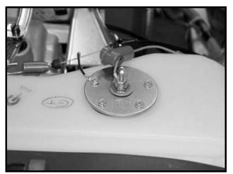
Figure 13a-9 Fuel Level Sensor
