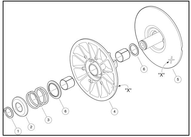
Figure 13b-39 Driven Clutch Assembly
