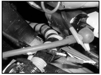
Figure 12a-3 Carburetor Coil Bullet Connector
