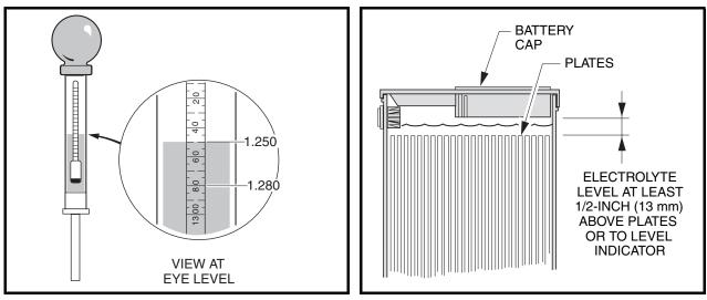
Figure 11b-3 Hydrometer Test
