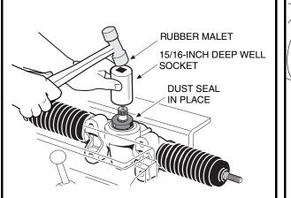
Figure 7-17 Press In Dust Seal
