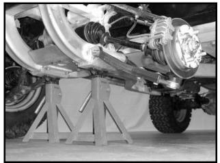
Figure 14-1 Place Jack Stands Under A-Frame Plates
