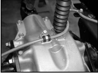
Figure 14-13 Receiver Hitch Brake Line T-Fitting and Bracket
