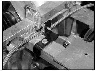
Figure 6-19 Front Brake Line T-Bracket
