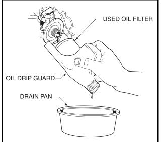
Figure 10-10 Remove Engine Oil Filter
