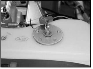
Figure 13b-19 Fuel Level Sensor
