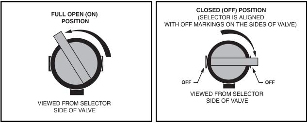
Figure 3-4 Fuel Shut-Off Valve – Open Position
