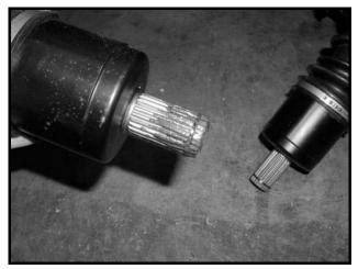
Figure 14-7 Apply Anti-Seize to Splined Ends
