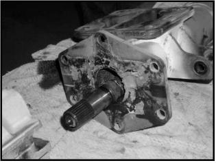
Figure 14-25 Separate Axle Tube from Differential
