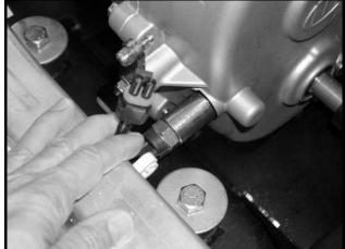
Figure 14-19 Neutral Sensing Connector
