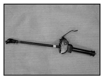
Figure 7-3 Steering Column Assembly
