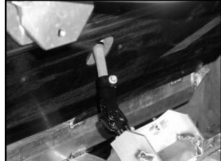
Figure 7-4 Steering Universal Joint
