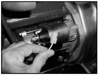
Figure 13b-6 Starter Solenoid Wire Connector
