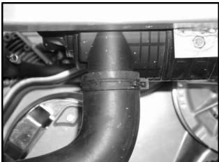
Figure 13a-30 Air Filter Inlet Hose
