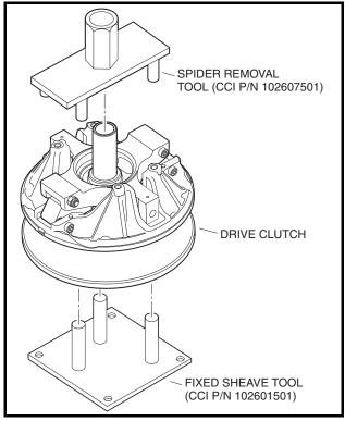
Figure 13a-33 Drive Clutch Service Tools
