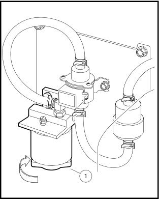
Figure 13b-13 Fuel Filter/Water Separator
