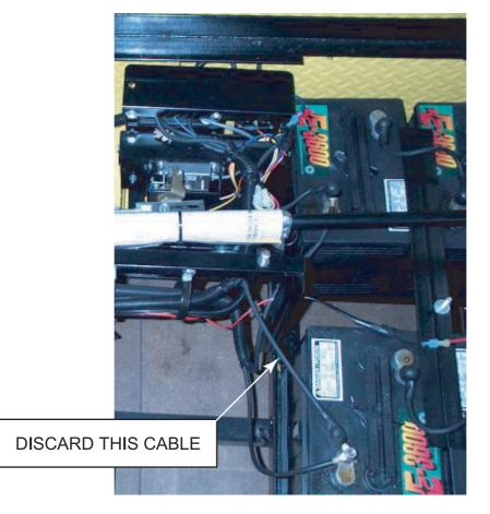
5. Fit new cable supplied with kit from a new switch terminal to the solenoid, ensuring that the fitted resistor is at the switch end from the solenoid. Make sure that all terminals are refitted to the solenoid.
