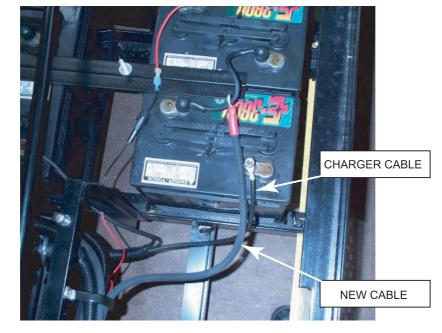
8. Connect new cable and charger cable to positive battery terminal.
