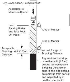
Typical Brake Performanace Test
