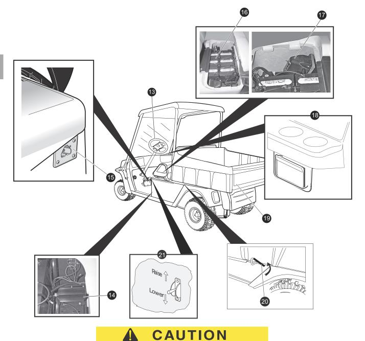
Before attempting to tow vehicle, move the Run-Tow/Maintenance switch to the 'Tow/Maintenance' position. Failure to do so will damage the controller or motor.
