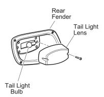
To replace the tail and brake light bulb, roll the rubber bezel from around the edge of the taillight and remove lens. Install replacement bulb and replace lens. To replace the tail and brake light bulb, remove hardware securing lens and remove lens. Install replacement bulb.
