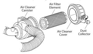
If the element is in acceptable condition, loose dirt may be removed by tapping the filter lightly. Do not use oil on the filter element or any part of the unit.
