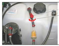
Fuel Shut-off Valve Turn to "OFF" Position
