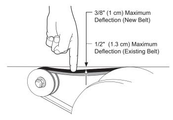
A **new** belt may be checked manually. A maximum deflection of 3/8" (10 mm) is acceptable. Tighten an **existing** belt to 75 - 80 lbs. (34 - 36 kg) tension using the same technique and inspect for cracking or wear. A maximum deflection of 1/2" (13 mm) is acceptable.
