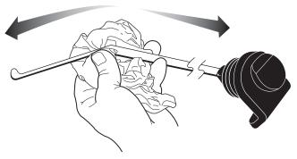
Insert the dipstick fully into the dipstick hole and remove. Examine the level of the oil on the dipstick.
