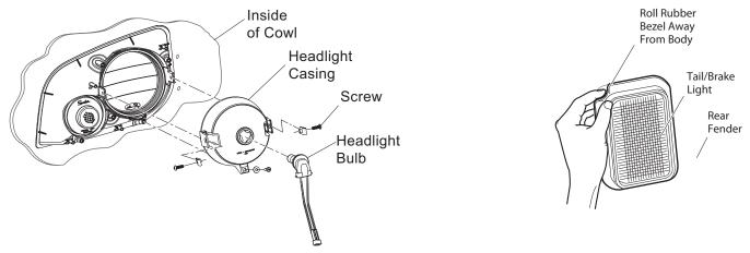
To replace the tail and brake light bulb, roll the rubber bezel from around the edge of the taillight and remove lens. Install replacement bulb and replace lens.
