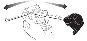
Insert the dipstick fully into the dipstick hole and remove. Examine the level of the oil on the dipstick.
