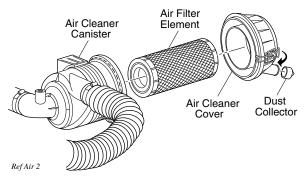
If the element is in acceptable condition, loose dirt may be removed by tapping the filter lightly. Do not use oil on the filter element or any part of the unit.
