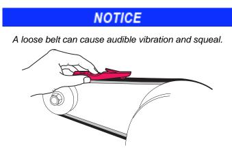
Tighten a **new** starter/generator belt to 115 - 125 lbs. (52-57 kg) tension when a gauge is applied half way between the two pulleys.
