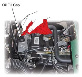
Fig. 36 Cleaning Top of Engine
