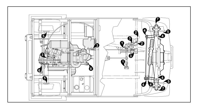
Figure 24 Lubrication Points – Gasoline Vehicles
