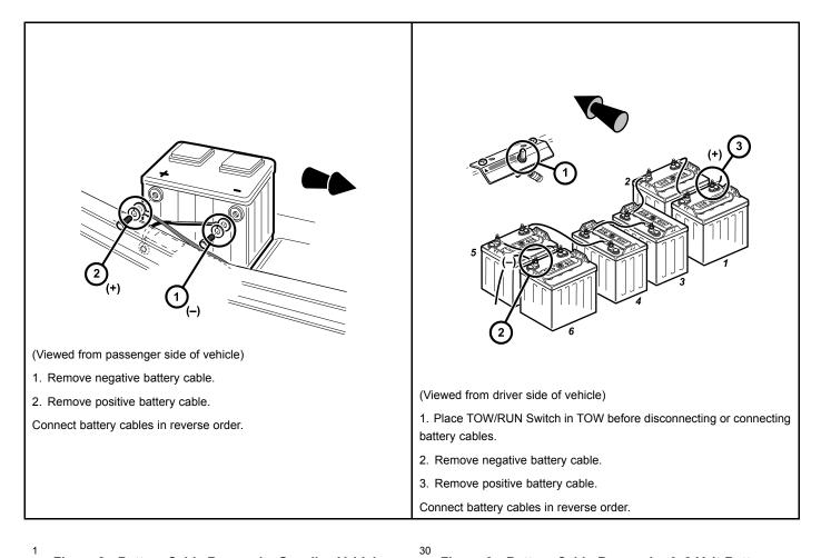
Figure 2 Battery Cable Removal – Gasoline Vehicle
