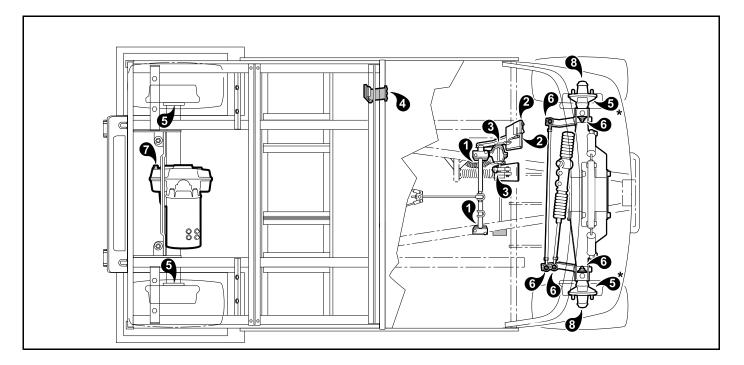
Figure 23 Lubrication Points – Electric Vehicles
