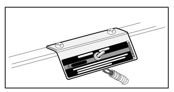
Figure 14 Tow/Run Switch – IQ System
