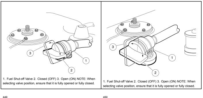
Figure 21 Fuel Shut-off Valve – 49-State Fuel Tank
